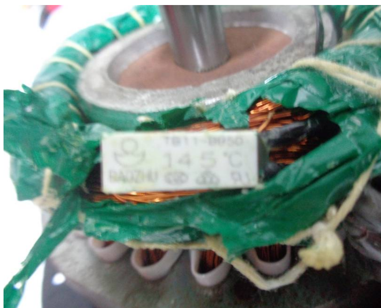
Figure 16 (Internal construction –thermal link of motor)
