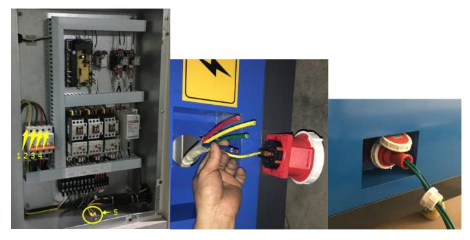
Push Male plug into Female plug. Push in till the end. Screw the locker to tighten the plugs.
