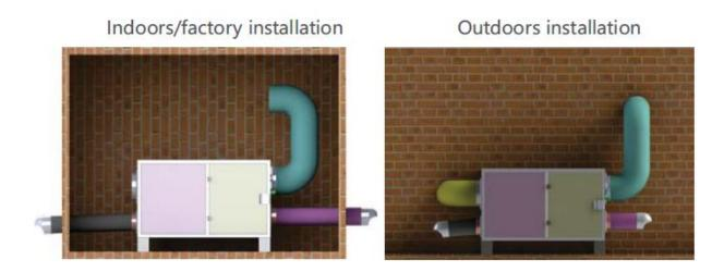
LUKO Desiccant Dehumidifier is design for easy ducting connection. For inspection and maintenance, please ensure there are enough space in front of the unit. This is to provide clearance for opening the access door and remove the desiccant wheel.
